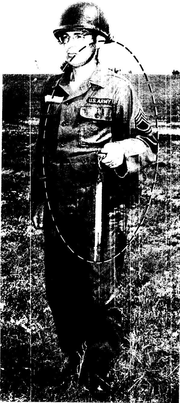
Figure 37. Ventilation of psychrometer.
